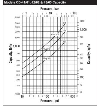
Capacities given are continuous discharge capacities in pounds and kilograms of hot condensate per hour at pressure differential indicated with condensate temperatures approximately 25°F (14°C) below steam temperatures.
